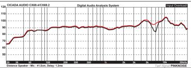
These are REAL frequency response curves of our CICADA AUDIO CoAx Speakers CX series. Typically Full-Range drivers sensitivity is measured full spectrum from 300Hz to 3kHz +/- 3dB (EIA standard) And "averaged". As you can see on the RTA curves these speakers average in the mid 90dB range with peaks over 100dB. The Black line indicates the frequency response of the same tweeter with AND without DPSH<sup>®</sup> "Dual-Phase Slot Horn". RED Line is WITH DPSH<sup>®</sup>. 10dB improvement!!
