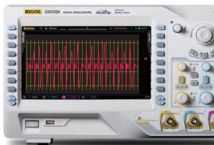
SCOPE LOOKING AT AC WAVEFORM OF MUSIC (HARD CLIPPED)
