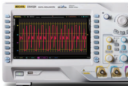
SCOPE LOOKING AT AC WAVEFORM OF MUSIC (HARD CLIPPED)
